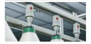
Simplified selection system helps to change the required brake force for various process parameters with out stopping the machine.
